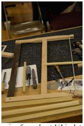
Traditional bow saws can be used for straight or curved cuts, with blades ranging from about 1/4 inch to an inch or more in depth, with the blade tensioned by the frame. Thus, it's also often described as a frame saw as well as a bow saw. "Bow saw" comes from the fact that more modern versions are made with a one-piece metal frame in a bowed shape. Chuck made the traditional wood-framed saw for us this evening.
