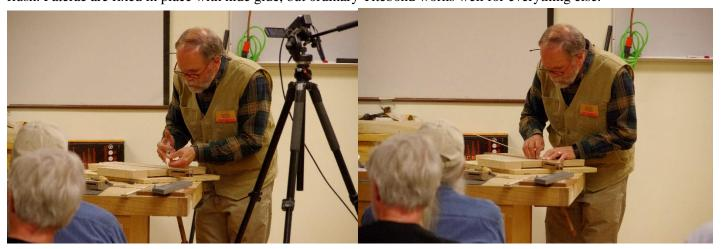
Rich has a variety of cutters for milling curved grooves and bends the strings to fit the required profile with a bit of heat. He expends considerable effort in trimming the corner joints, especially where curved strings intersect straight ones, using chisels and plane irons and incredible patience to get perfect joints.
