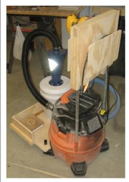
on top of a five gallon plastic pail and that could make the shop vac more difficult to move about. The solution that I came up with was a small platform attached to the shop vac. The platform has a single dolly wheel under it to keep it all level and portable.
