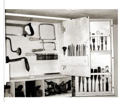
has planes chisels, rifflers and rasps in front with saws hanging inside the cabinet. This cabinet has screw drivers, pliers, nut driverssquares, and measuring tapes... plus the drawers. With doors closed the hand saws and framing squares fit
